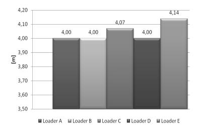
Fig. 1. Maximum lifting height of bucket pivot points in front-end loaders
