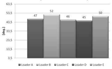
Fig. 4. Material loading angle of front-end loaders
