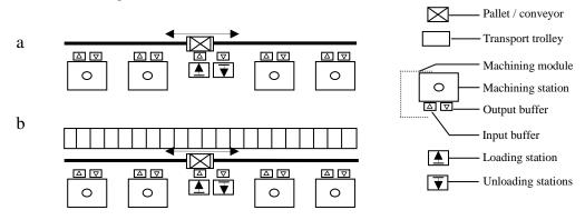
Fig. 2. Diagram of a flexible manufacturing system with central transport between stations (a) and with a central production warehouse (b)
