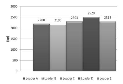
Fig. 2. Front-end loader lifting capacity at minimum height
