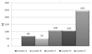
Fig. 8. Front-end loader disassembling time
