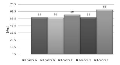
Fig. 5. The angle at maximum height during unloading in front-end loaders
