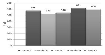
Fig. 6. Mass of front-end loaders
