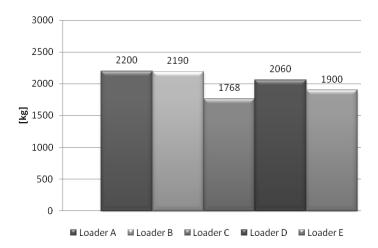
Fig. 3. Front-end loader lifting capacity at maximum height
